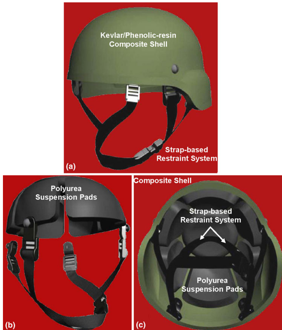
Fig. 1 The advanced combat helmet (ACH): (a) external side view, (b) suspension system side view, and (c) suspension system bottom view
